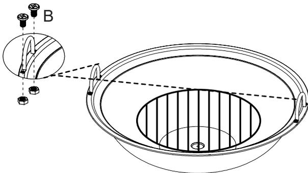
6- Mount the spark screen to the upper section of the smokestack using 2 small screws with washers.
