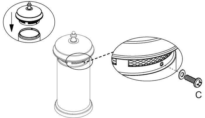
8 - Mount the smokestack to the upper heat and smoke shield. Fit down snug then slowly twist counterclockwise until all 4 tabs lock securely in place.
