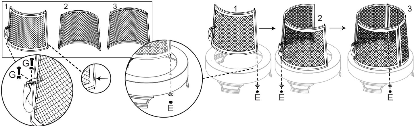
3- Fasten the screens together with the screws and washers, be sure to get the top and the bottom.
