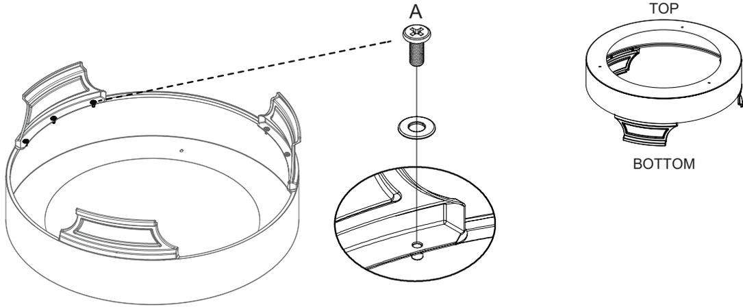
2- Turn the base over and assemble the upper mesh screens onto the base. Each screen has a screw that goes in the hole in the base with 2 tabs to connect to the adjacent screen using screws. The screens can start in any hole, but it is easiest to start with the screen that has the hinge for the door first and install the frame with the door last.
