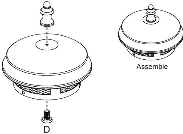
7 - Assemble the smokestack. Be sure that all 3 tabs of the upper section lock in place with the lower section. Be sure to twist counterclockwise and twist until it locks securely.
