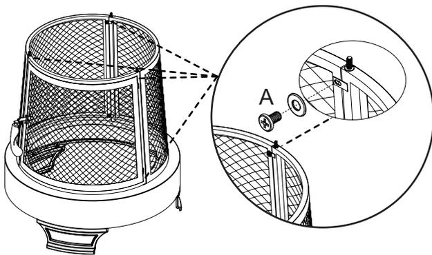
4- Connect the top heat and smoke shield to the body. Be careful to not damage the threads of the bolts when installing. There are three mounting points. Reach down through the top and use as washer and nut on each screw to fasten.
